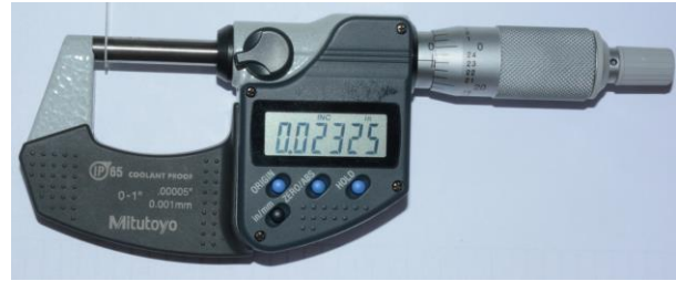
Figure 2: Micrometer used to take digital readout in inches
